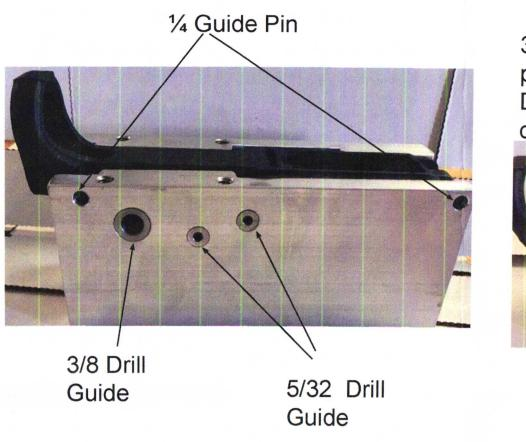
3/8 Drill in 2 places Drill to 630 depth 630 for a constraint of the second sec
