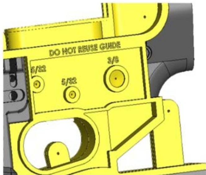
WITH THE JIG PLACED FLAT ON ONE SIDE, USE A 3/8" DRILL BIT TO DRILL THE SAFTEY SELECTOR HOLE AND A 5/32" BIT TO DRILL THE TRIGGER AND HAMMER PIN HOLES. DO NOT DRILL THESE HOLES ALL THE WAY FROM ONE SIDE TO THE OTHER. DRILL ONE SIDE THEN FLIP THE JIG AND DRILL THE OTHER. REMOVE THE LOWER FROM THE JIG AND FINISH BY DEBURRING WITH A SMALL FILE.
